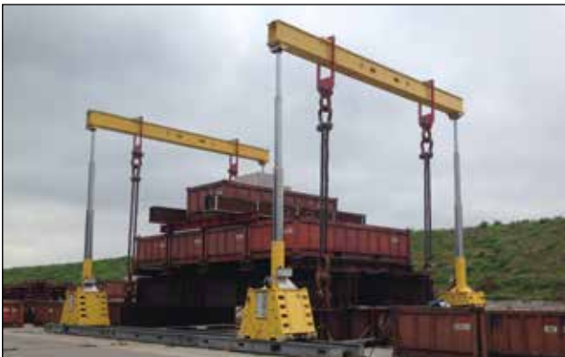
◀ SL-400 Series Gantry during load testing.
